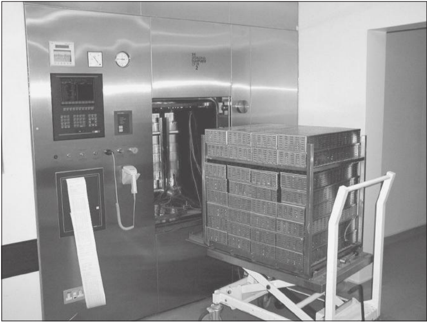
Figure 6.3 Autoclave at Pharmacy Manufacturing Unit, Torbay Hospital.
