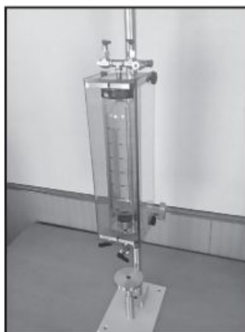
Fig. 8.4: Pressure burettes for filling aerosols
